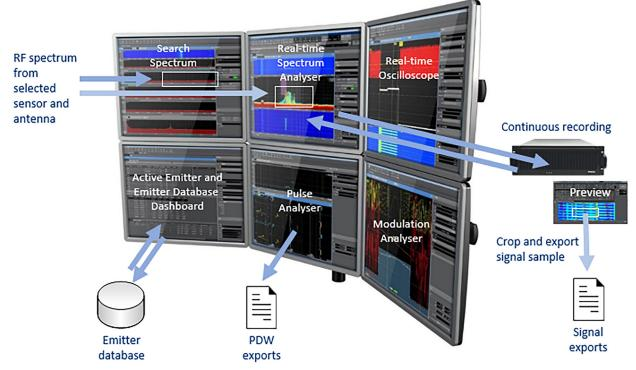
To analyse a chosen waveform in more detail, signals can be detected from a chosen sub-band and illustrated with real-time oscilloscope displays. These can be used to analyse intra-pulse and interpulse modulations or e.g. beam patterns.
